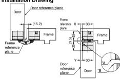
\*The door and frame need to be chamfered based on the machining margin
