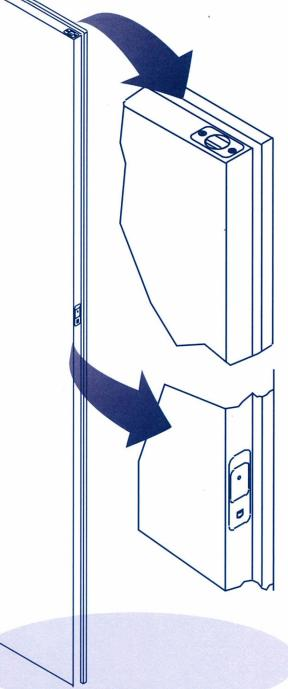
Push & Go Evo magnetic flush bolt is designed to release the inactive leaf of a double door at the push of a button.
