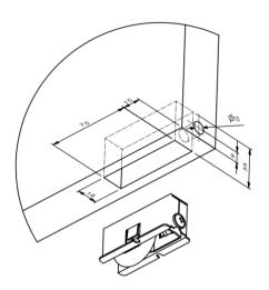
NOTE – carriages are a press fit. Tabs on side of carriage hold the unit in place. Optional screw hole situated at the top of carriage between wheel and adjustment screw if required.
